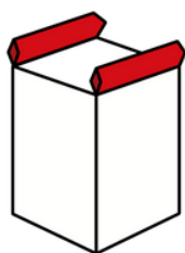
Tunnel Loops (Sleeve Lifting)
